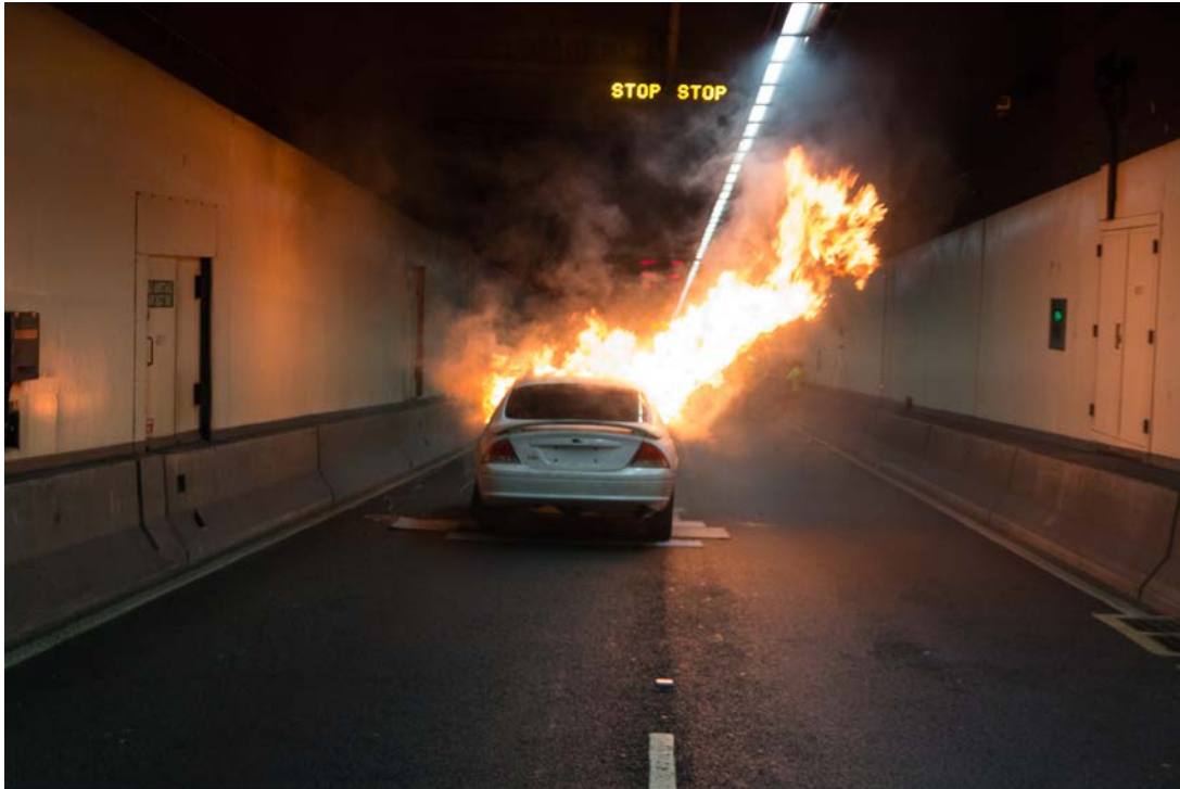
Figure 2-45: Sydney Harbor Tunnel live fire and FFFS demo, prior to FFFS activation.
