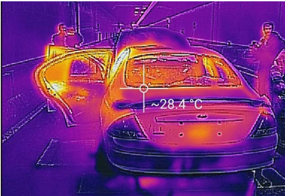
Figure 2-54: Sydney Harbor Tunnel live fire and FFFS demo, post-test view of vehicle, thermal heat map
