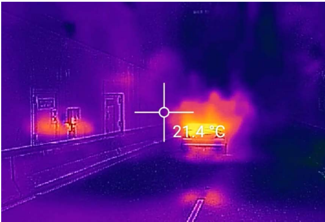
Figure 2-50: Sydney Harbor Tunnel live fire and FFFS demo about 1 minute after FFFS activation, thermal heat map.
