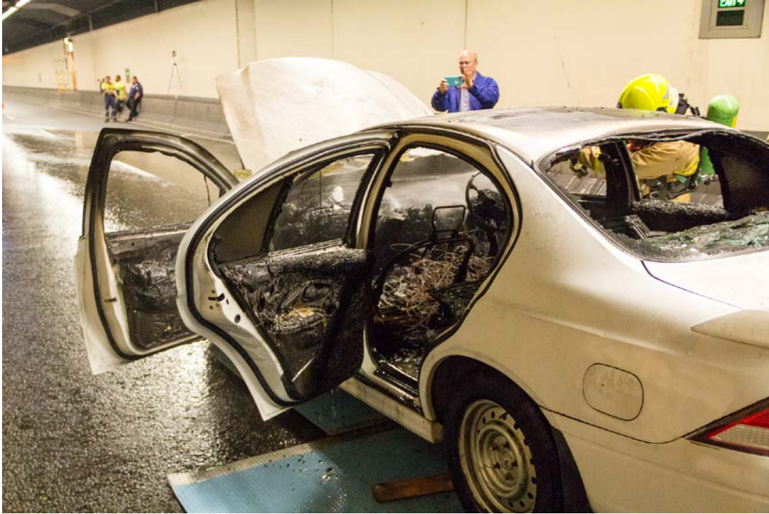
Figure 2-53: Sydney Harbor Tunnel live fire and FFFS demo, post-test view of vehicle.
