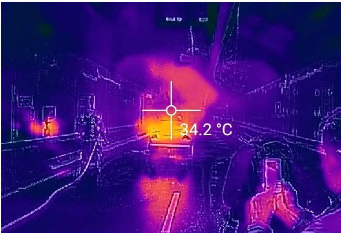
Figure 2-52: Sydney Harbor Tunnel live fire and FFFS demo during fire brigade intervention, thermal heat map.
