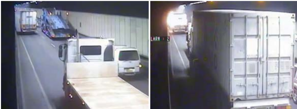
Figure 2-42: M5 East fire inside of tunnel, start of incident 00:00 (left) and visible flame at 03:00 (right).
