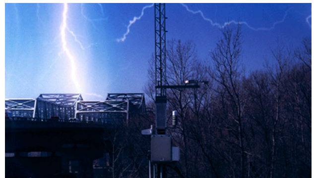
FIGURE 3. ENVIRONMENTAL SENSOR STATION. SOURCE: VAISALA
