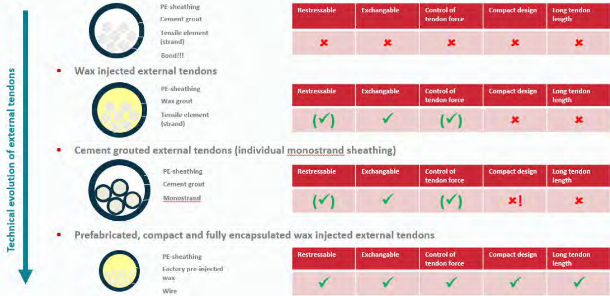
Figure 21: This table details the various external tendon and filling types along with the potential advantages and drawbacks of each (Source: DYWIDAG)
